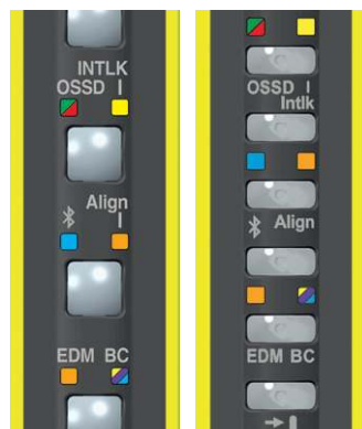
FIG. 8B: LED INDICATORS ON RECEIVER UNIT (30 MM AND 14 MM RESOLUTION)
