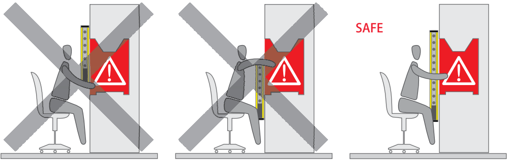
FIG. 9: POSITIONING THE LIGHT CURTAIN
